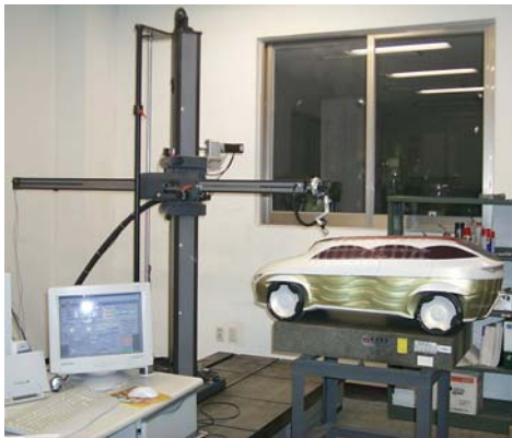
Fig. 1. Layout machine for 3D digitizing.
